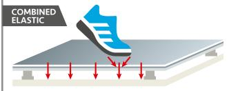
A combination of an area elastic system with a point elastic top surface. Deformation over both a small area in the point elastic and large area in the area elastic layers.
