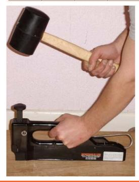
AF Mallet Drive Spotnailer. In production for over 65 years, still a reliable method of laying hardboard. The specially developed narrow crown is automatically countersunk below the surface. This tool needs no power source to work, just take it out of your toolbox and use. The staples are 18 gauge galvanized, with diversion chisel points for maximum hold. This staple was developed in conjunction with the trade, especially for flooring.
